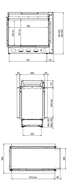
For the e-MatriX series, whilst stocks last, the fire casing may be 32mm lower than noted on the drawings in these brochures. After delivery, check the height of the fire casing to prevent misunderstandings.
